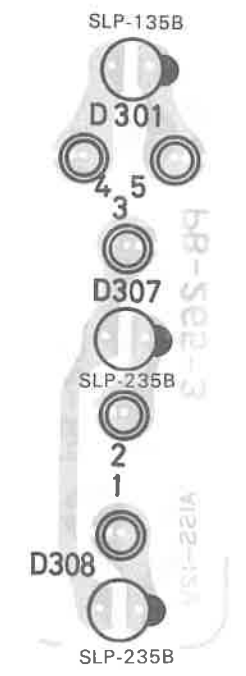
LED INDICATOR P.C.B. BOTTOM VIEW
