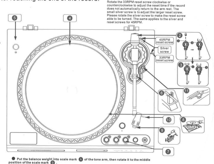
Rotate the balance weight counterclockwise so that it moves outward towards position 📵
